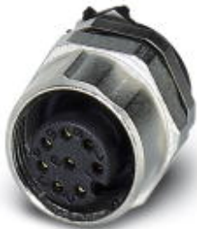
Sensor/actuator flush-type connector, socket, 8-pos., M12 SPEEDCON, A-coded, shielded, rear/screw mounting with M12 thread, with straight THR solder connection
