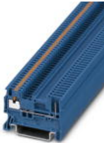
Feed-through terminal block, Connection method: Push-in / plug connection, Cross section: 0.14 mm 2 - 1.5 mm 2 , AWG: 26 - 16, Width: 3.5 mm, Color: blue, Mounting type: NS 35/7,5, NS 35/15
