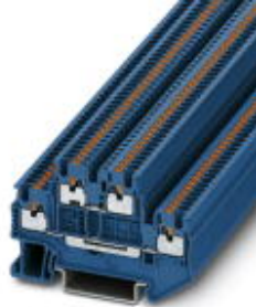
Double-level terminal block, Cross section: 0.14 mm 2 - 1.5 mm 2 , AWG: 26 - 14, Connection type: Push-in connection, Width: 3.5 mm, Color: blue, Mounting type: NS 35/7,5, NS 35/15
