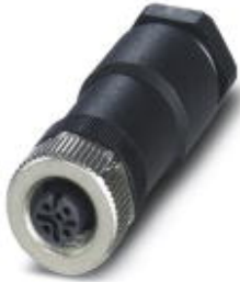
Connector, Universal, 4-position, Socket straight M12, A-coded, Screw connection, Knurl material: Zinc die-cast, nickel-plated, Cable gland Pg11, External cable diameter 8 mm ... 10 mm
