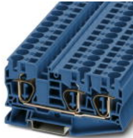
Feed-through terminal block, Connection method: Spring-cage connection, Cross section: 0.2 mm 2 - 16 mm 2 , AWG: 24 - 6, Width: 10.2 mm, Color: blue, Mounting type: NS 35/7,5, NS 35/15
