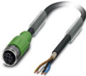
Sensor/Actuator cable, 4-position, PUR halogen-free, Black-gray RAL 7021, shielded, Free cable end, on Socket straight M12, A-coded, Cable length: 5 m
