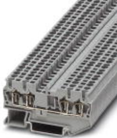
Feed-through terminal block, Connection method: Spring-cage connection, Cross section: 0.08 mm 2 - 4 mm 2 , AWG: 28 - 12, Width: 5.2 mm, Color: gray, Mounting type: NS 35/7,5, NS 35/15
