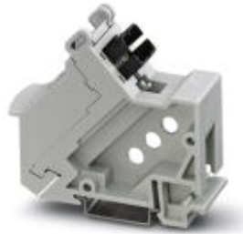
Patch panel, SCRJ, DIN rail mounting, IP20, 1 slot, socket/socket, can be used for glass, multi-mode, HCS, and polymer fibers
