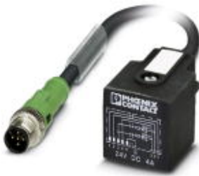
Sensor/Actuator cable, 5-position, PUR halogen-free, Black-gray RAL 7021, Plug straight M12, A-coded, on Valve connector AD (pressure switch), with 2 LEDs, Cable length: 1.5 m
