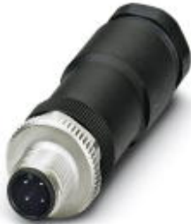
Sensor/actuator connector, male, straight, 4-pos., M12, A-coded, screw connection, metal knurl, cable screw connection Pg11-DUO
