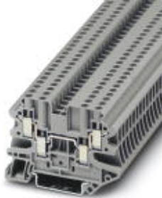
Feed-through terminal block, Connection method: Screw connection, Cross section: 0.14 mm 2 - 4 mm 2 , AWG: 26 - 12, Width: 5.2 mm, Color: gray, Mounting type: NS 35/7,5, NS 35/15
