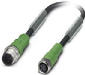
Sensor/Actuator cable, 3-position, PUR halogen-free, Black-gray RAL 7021, Plug straight M12, A-coded, on Socket straight M8, Cable length: 0.6 m
