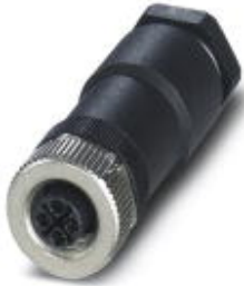
Connector, Universal, 4-position, Socket straight M12, S-coded, Screw connection, Knurl material: Zinc die-cast, nickel-plated, Cable gland Pg11, External cable diameter 8 mm ... 10 mm
