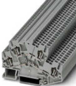
Feed-through terminal block, Cross section: 0.08 mm 2 - 4 mm 2 , AWG: 28 - 12, Connection type: Spring-cage connection, Width: 5.2 mm, Color: gray, Mounting type: NS 35/7,5, NS 35/15
