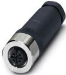
Sensor/actuator connector, female, straight, 5-pos., M12, screw connection, high-grade steel knurl, cable screw connection Pg9
