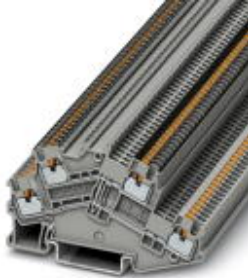
Double-level terminal block, Cross section: 0.14 mm 2 - 1.5 mm 2 , AWG: 26 - 14, Connection type: Push-in connection, Width: 3.5 mm, Color: gray, Mounting type: NS 35/7,5, NS 35/15
