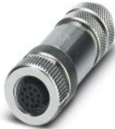
Connector, Universal, 12-position, shielded, Socket straight M12, A-coded, Solder connection, Knurl material: Zinc die-cast, nickel-plated, Cable gland Pg9, External cable diameter 6 mm ... 8 mm
