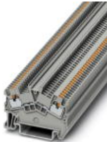
Feed-through terminal block, Connection method: Push-in connection, Cross section: 0.14 mm 2 - 1.5 mm 2 , AWG: 26 - 14, Width: 3.5 mm, Height: 37 mm, Color: gray, Mounting type: NS 35/7,5, NS 35/15
