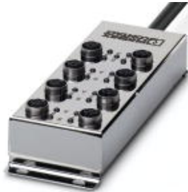
Sensor/actuator box, M12 socket, 8 slots, 5-pos., double occupancy, status indicator: yes, pnp, master cable connection: Fixed connection 180°, PVC, cable length: 10 m, shielding: No
