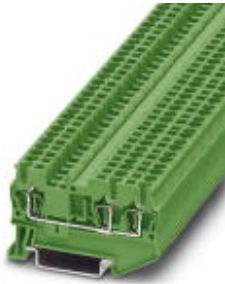
Feed-through terminal block, Connection method: Spring-cage connection, Cross section: 0.08 mm 2 - 4 mm 2 , AWG: 28 - 12, Width: 5.2 mm, Color: green, Mounting type: NS 35/7,5, NS 35/15
