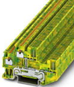
Protective conductor double-level terminal block, Cross section: 0.14 mm 2 - 1.5 mm 2 , AWG: 26 - 16, Connection type: Push-in / plug connection, Width: 3.5 mm, Color: green/yellow, Mounting type: NS 35/7,5, NS 35/15
