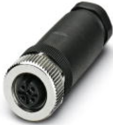
Sensor/actuator connector, female, straight, 4-pos., M12, A-coded, screw connection, metal knurl, cable screw connection Pg9
