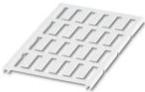
Snap-in markers, Sheet, white, Unlabeled, Can be labeled with: BLUEMARK CLED, BLUEMARK LED, Plotter, Mounting type: Snapped into marker carrier, Lettering field: 20 x 7 mm
