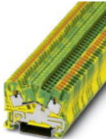
Ground modular terminal block, Connection method: Push-in connection, Cross section: 0.14 mm 2 - 4 mm 2 , AWG: 26 - 12, Width: 5.2 mm, Color: green-yellow, Mounting type: NS 35/7,5, NS 35/15
