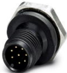
Sensor/actuator flush-type connector, male, 8-pos., M12, A-coded, front/screw mounting with M16 thread, with solder cups, plastic version
