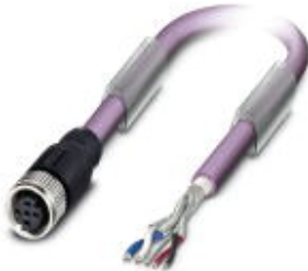
Bus system cable, CANopen ® , DeviceNet ™ , CANopen ® /DeviceNet ™ , 5-position, PUR halogen-free, Violet, RAL 4001, shielded, Free cable end, on Socket straight M12, A-coded, Cable length: 2 m
