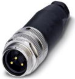
Sensor/actuator connector, male, straight, 3-pos., 7-8", screw connection, metal knurl, cable screw connection Pg9
