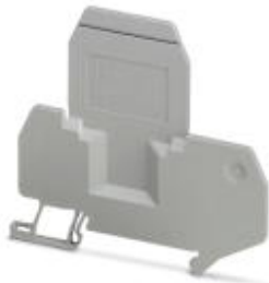
Partition plate, Length: 74.3 mm, Width: 2.2 mm, Height: 70 mm, Color: gray
