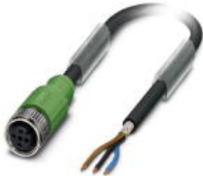
Sensor/Actuator cable, 3-position, PUR halogen-free, Black-gray RAL 7021, shielded, Free cable end, on Socket straight M12, A-coded, Cable length: 10 m
