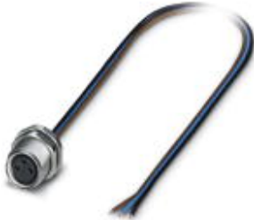
Sensor/actuator flush-type socket, 3-pos., M8, rear/screw mounting with M10 thread, with 0.5 m TPE litz wire, 3 x 0.25 mm²
