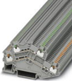
Component terminal block, Cross section: 0.14 mm 2 - 1.5 mm 2 , AWG: 26 - 14, Connection type: Push-in connection, Width: 3.5 mm, Color: Green/orange, Mounting type: NS 35/7,5, NS 35/15
