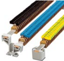
Connection terminal block, Connection method Screw connection, Load current : 41 A, Cross section: 0.5 mm 2 - 6 mm 2 , Width: 7 mm, Color: green-yellow
