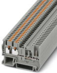
Feed-through terminal block, Connection method: Push-in / plug connection, Cross section: 0.14 mm 2 - 4 mm 2 , AWG: 26 - 12, Width: 5.2 mm, Height: 35.2 mm, Color: gray, Mounting type: NS 35/7,5, NS 35/15
