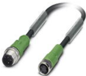
Sensor/Actuator cable, 3-position, PUR halogen-free, Black-gray RAL 7021, Plug straight M12, A-coded, on Socket straight M8, Cable length: 5 m
