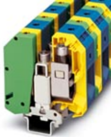
Ground modular terminal block, Screw connection, Cross section: 25 mm 2 - 95 mm 2 , AWG: 3 - 3/0, Width: 50 mm, Color: green-yellow, Mounting type: NS 35/15, NS 32
