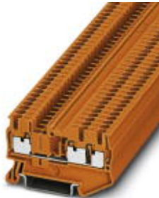
Feed-through terminal block, Connection method: Push-in connection, Cross section: 0.14 mm 2 - 4 mm 2 , AWG: 26 - 12, Width: 5.2 mm, Color: orange, Mounting type: NS 35/7,5, NS 35/15
