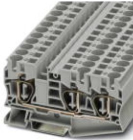
Feed-through terminal block, Connection method: Spring-cage connection, Cross section: 0.2 mm 2 - 16 mm 2 , AWG: 24 - 6, Width: 10.2 mm, Color: gray, Mounting type: NS 35/7,5, NS 35/15
