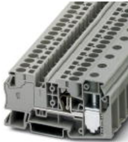
Feed-through terminal block, Connection method: Screw connection, Cross section: 1.5 mm 2 - 50 mm 2 , AWG: 16 - 1/0, Width: 16.2 mm, Color: gray, Mounting type: NS 35/7,5, NS 35/15
