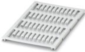
Conductor marker, Sheet, white, Unlabeled, Can be labeled with: BLUEMARK CLED, BLUEMARK LED, Plotter, Mounting type: Slide on, Cable diameter: 1.6-2.1 mm, Lettering field: 12 x 3 mm
