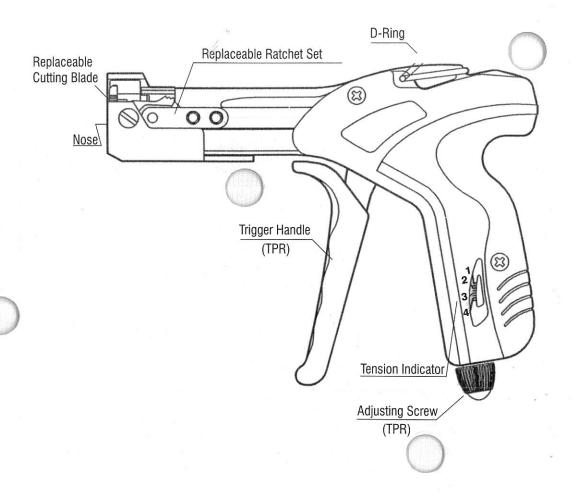
For cable tie thickness up to 0.3mm. width up to 7.9mm steel plate
