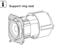
The support ring of the loudspeaker insert is coated with a film that provides acoustic isolation of the insert from the front sound opening. This support ring seal **must not be removed** and, apart from holes caused by the attachment screws must **not be damaged**, as otherwise bass reproduction may be impaired.
