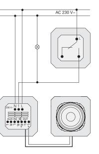
If no permanent phase exists in the room, connection of the flush-mounted radio can alternatively be carried out via the switched phase. In this case however the flush-mounted radio may only be operated with lighting switched on.
