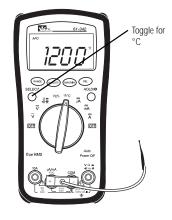
NARNING: To avoid electric shock, do not place test leads or thermocouple on a voltage source.
