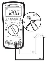
MARNING: De-energize circuit before taking resistance measurement.
