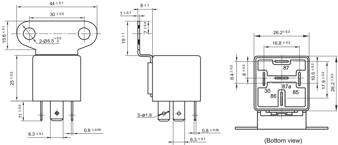
Remark: Terminal vertical deviation tolerance is 0.3mm.
