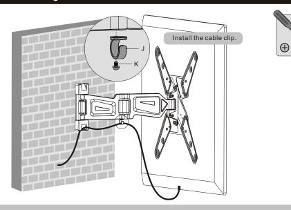
Connect the cables to your TV and route the cables through the cable clip. Note: Leave slack in the cable for cantilever arm movement.
