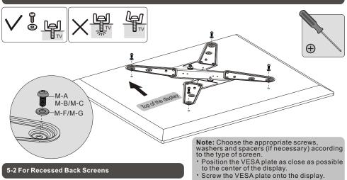
Tighten all screws but do not over tighten.
