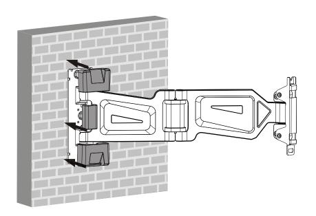
Install the decorative covers along the wall plate rail until they fit snugly onto the wall plate.
