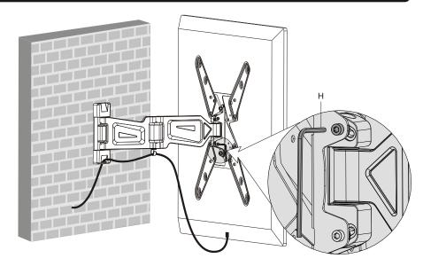
It is necessary to slightly loosen or tighten the adjustment screws using an Allen key according to the weight of TV installed.
