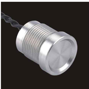
647848 : Piezo switch, flux16mm, 4.5mm finger location operator, Aluminium, 200mA, 24 V AC/DC
