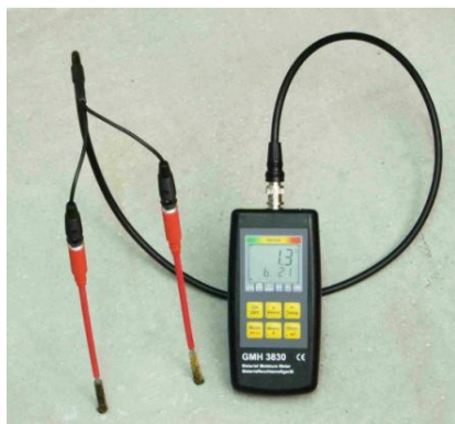
Measuring with brush probe GBSL91
