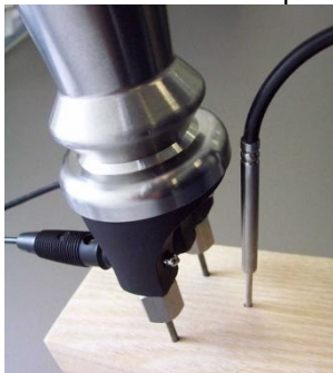
Reciprocating piston electrode GHE91 with temperature-probe GTF38
