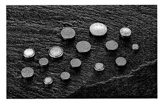
Silver oxide is used as cathode, zinc is used as anode, and sodium hydroxide solution or pottasium hydroxide solution is used as electrolyte. These batteries with large capacity and stable voltage characteristics are widely applied to products demanding high accuracy, like quartz watches.
