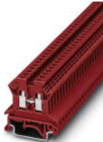
Feed-through terminal block, Connection method: Screw connection, Cross section: 0.2 mm 2 - 4 mm 2 , AWG: 24 - 14, Width: 5.2 mm, Color: red, Mounting type: NS 35/7,5, NS 35/15
