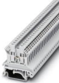
Feed-through terminal block, Connection method: Screw connection, Cross section: 0.2 mm 2 - 4 mm 2 , AWG: 24 - 14, Width: 5.2 mm, Color: white, Mounting type: NS 35/7,5, NS 35/15
