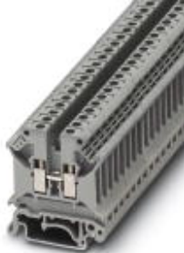
Feed-through terminal block, Connection method: Screw connection, Number of positions: 1, Cross section: 0.2 mm 2 - 6 mm 2 , AWG: 24 - 10, Width: 6.2 mm, Color: gray, Mounting type: NS 32, NS 35/7,5, NS 35/15
